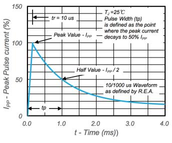
Fig.3 - Pulse Waveform
