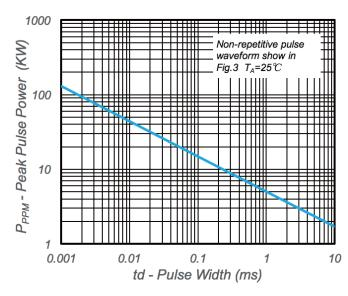
Fig.1 - Peak Pulse Power Rating
